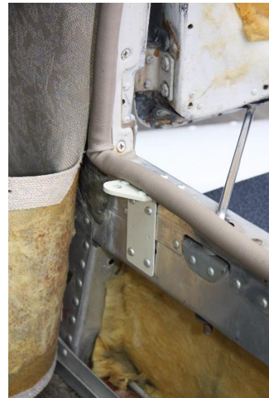
Figure 4. Bracket riveted, wind lace reinstalled between layers
