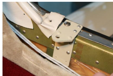
Figure 21. Airframe bracket attached (Note: bottom 2 pilot holes not used.)
