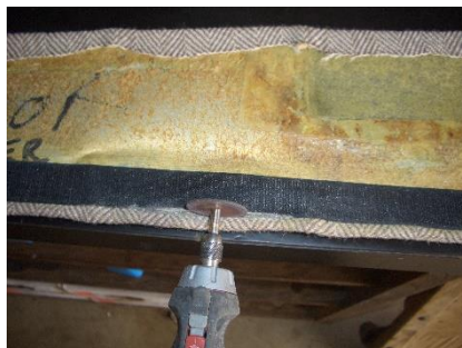
Figure 7. Slotting interior panel on Baron
