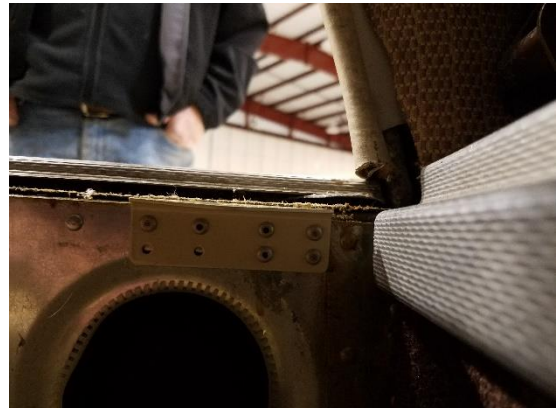
Figure 33. Airframe bracket attached to door sill
