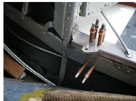
Figure 2 Airframe bracket clecoed in place
