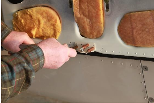
Figure 23. Installing Door Bracket
