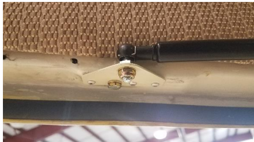
Figure 34. Gas spring attached to door
