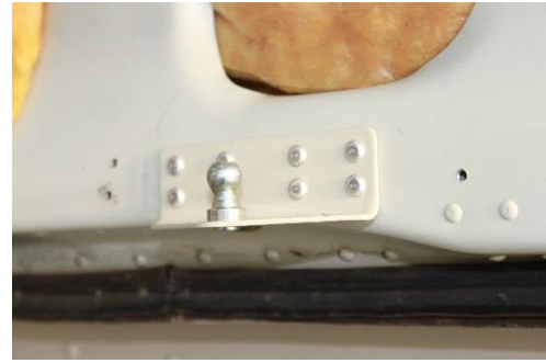
Figure 24. Door Bracket Installed
