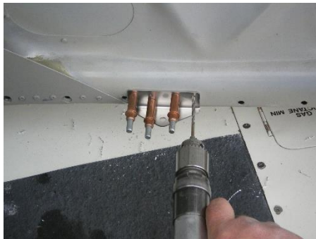
Figure 5. Drilling door bracket
